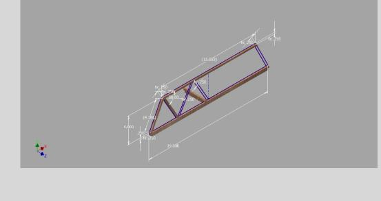
Identical frame members were only created once and then assembled multiple times in order to reduce errors. The final assembly has physical constraints assigned to each member defining joint attachments.
