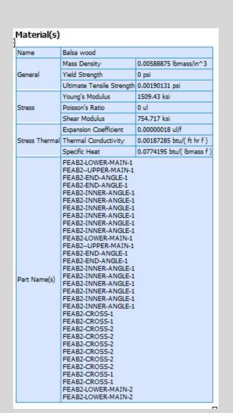
An average material was derived based from typical properties found through distributors.
